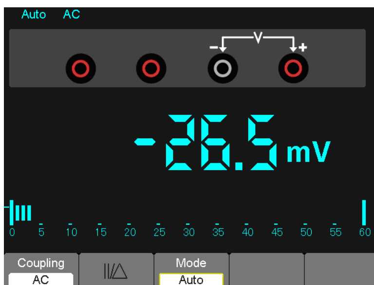
Figure 7-7 AC voltage Measurement
