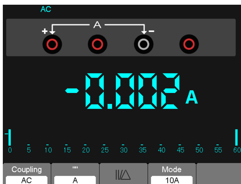
Figure 7-11 AC Current Measurement for 10A
