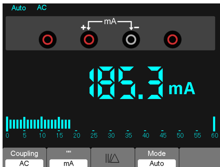
Figure 7-10 AC Current Measurement for 600 mA
