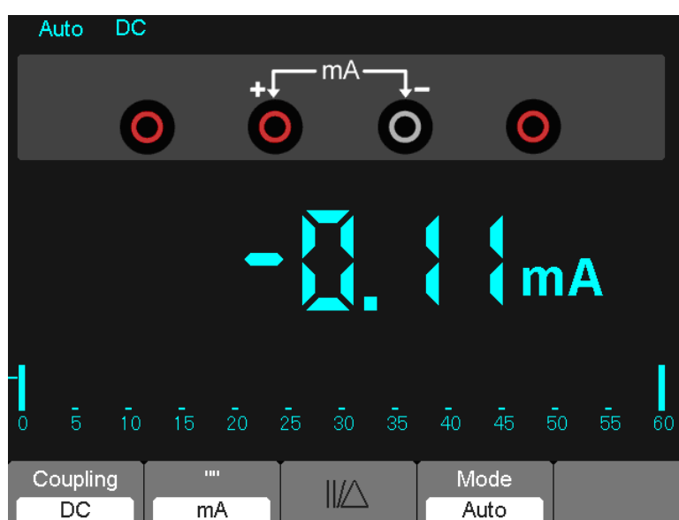
Figure 7-8 DC current Measurement for 600 Measurement
