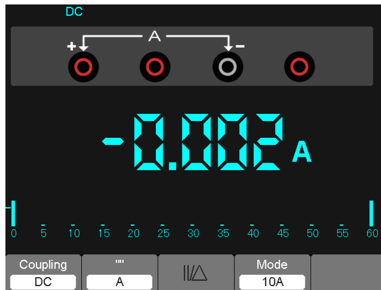
Figure 7-9 DC Current Measurement for 10A
