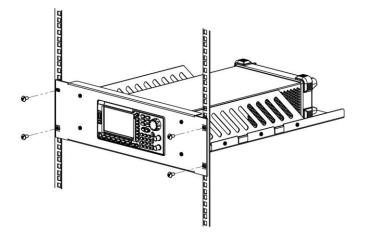
**7.** Post-installation notice: The rack occupies a height of 3U. The holes pointed out by the arrows are the installation holes. Note that they are aligned while installing.
