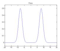
Note that, being different from the **Pulse** in basic waveform, the Pulse mentioned here can be configured by setting the parameters "Pulse Width/Duty Cycle", "Leading" and "Trailing".
