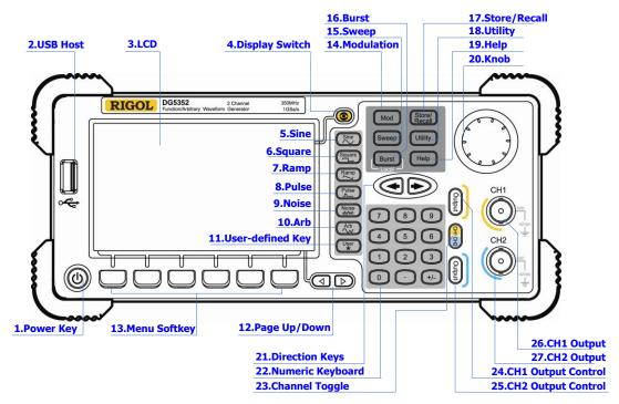
Figure 1-1 Dual-Channel Model Front Panel Overview
