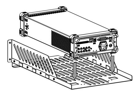
**4.** Fixed the instrument: Fasten the instrument tightly on the Support Board with two Fixed Figures and fixed it with four M4 screws.
