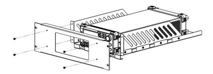
**6.** Load into the machine cabinet: mount the rack fixed with instrument into a standard 19-inch machine cabinet with four M6 screws and square nuts.
