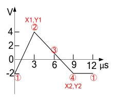
**Note:** As can be seen from the above figure, the waveform editor will automatically connect the last point to the voltage level of the first point to create a continuous waveform.
