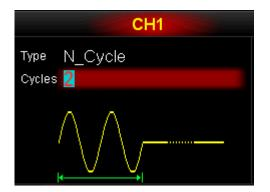
N Cycle Burst could be triggered by "Internal", "External" or "Manual" source. You can
