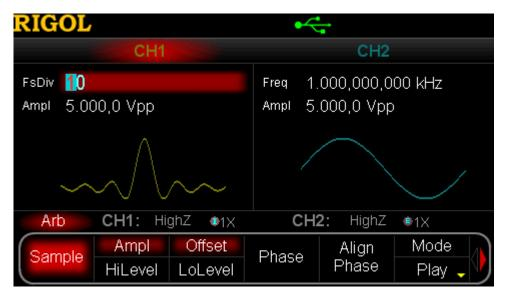
Figure 3-2 Arbitrary waveform output mode (Play)
