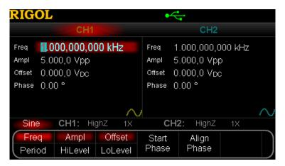
Figure 1-5 User Interface (Parameter Mode)
