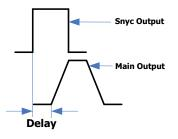
Press **Pulse**  $\rightarrow$  **Delay** to highlight the softkey, and then use the numeric keyboard to input "8" and select the unit " $\mu$ s" in the pop-up menu.
