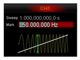
The generator will renewedly sweep and output with the specified "Start Frequency" once the Mark Frequency is changed.
