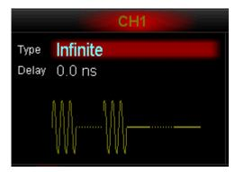
Infinite Burst could be triggered by "External" or "Manual" source. You can also set "**Start Phase**", "**Delay**", "**Trigger Input**" (external trigger) and "**Trigger Output**" (manual trigger).
