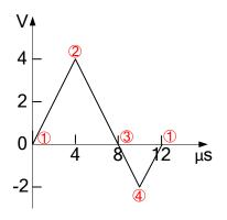
**Note:** As can be seen from the above figure, the waveform editor will automatically connect the last point to the voltage level of the first point to create a continuous waveform.
