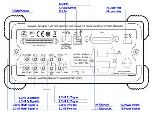
Figure 1-3 Dual-Channel Model Rear Panel Overview
