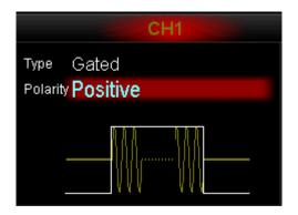
Gated Burst could only be triggered by "External" source. You can also set "Start Phase".
