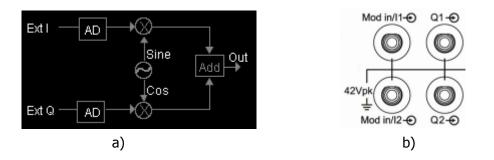
As shown in figure a), the external I and Q signals are sampled by the generator and then the IQ modulating signals are acquired.
