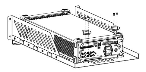
**5.** Install the Front Panel: aiming the instrument front panel at the opening of the Front Panel of the machine rack and fix them with four M4 screws.
