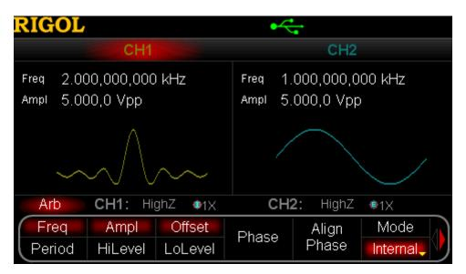
Figure 3-1 Arbitrary waveform output mode (Internal)
