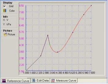
The last window is the Measure Curve. Here the real time measured waveform of the Digital Multimeter is displayed. The waveform can be replayed after it has been recorded and it can also be exported as a \*.txt or\*.csv file and so used as a future reference curve.
